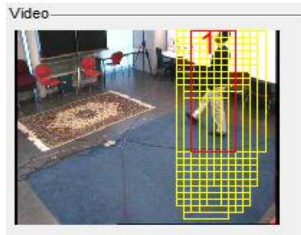
Figure 2. Detection and tracking of single moving object in frame t.
