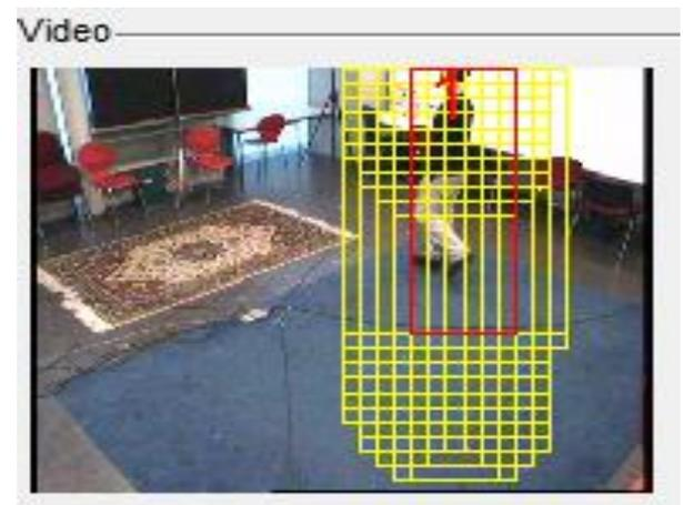
Figure 3. Detection and tracking of single moving object in frame t+1.
