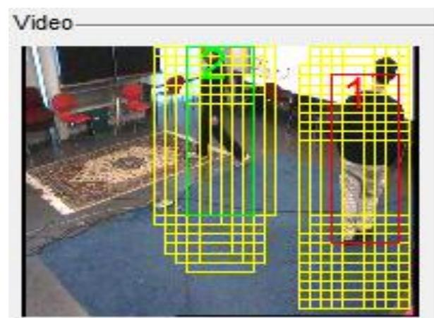
Figure 4. Detection and tracking of multiple moving objects in frame t.
