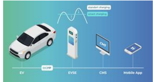
Fig. 4. Integrated central management system under OCPP protocol
