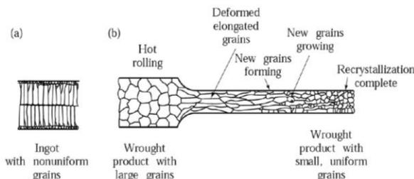
The process is illustrated in figure, which shows the changes that takes place in the grain structure of the
