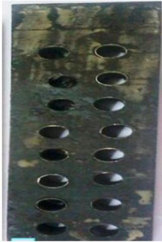
Fig 4 Drilled specimen of EN24 Steel
