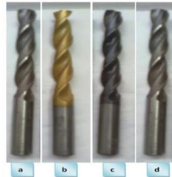
Fig 2 Drill bits (a) HSS (b) TiN coated HSS (c) HSS with 5% Cobalt (d) HSS with 8% Cobalt
